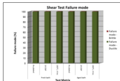
(b) Shear Force and Failure mode of the ENIG deposit of Conventional cyanide-containing immersion gold
