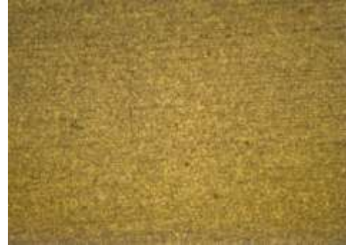
FIGURE 10. POROSITY TEST RESULT FOR NEW BATH
